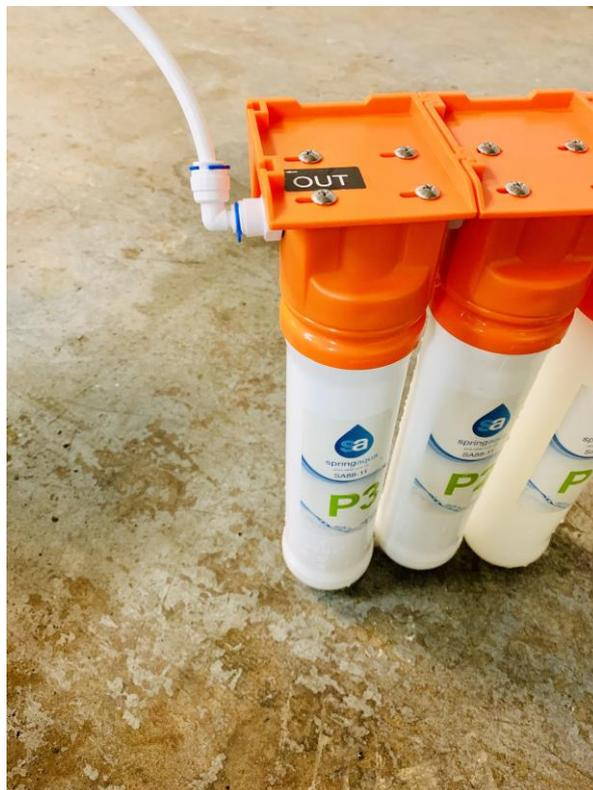
4. Turn the water on, make sure all the shut off valves are on, and flush the Pre Filter for 1 min. You will need to aim the white ¼ nylon pipe coming out of the pre filter “OUT” towards the sink so that the water is drained in the sink while flushing.
